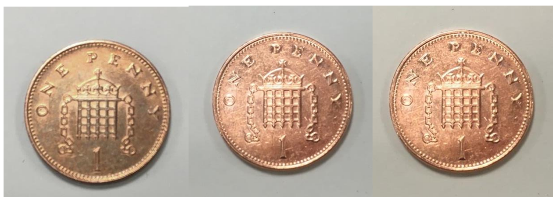
Figure 3.11: A) British 1 penny before HCl wash (dirty), B) British 1 penny after HCl wash (clean and shiny) and C) British 1 penny after polymerization was stopped (still clean and shiny). Neither B) nor C) shows any macroscopic physical damage, defacing or destruction to the coin.
