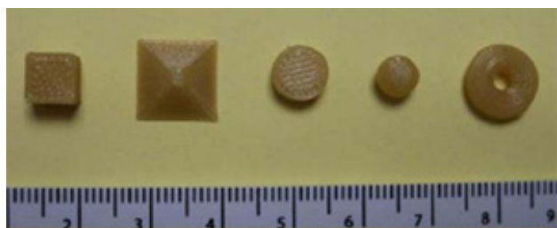
Figure 6. Cube, pyramid, cylinder, sphere and torus paracetamol tablets fabricated by Goyanes et al. 34
