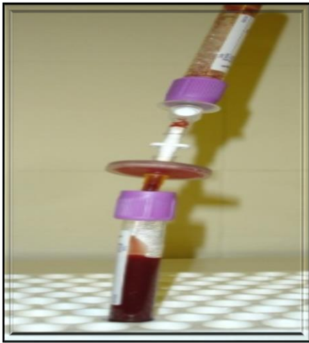
Figure 2-2: LeukoLOCK capture filter – 6ml sample of blood is passed through a LeukoLOCK filter, which captures the total leukocyte population
