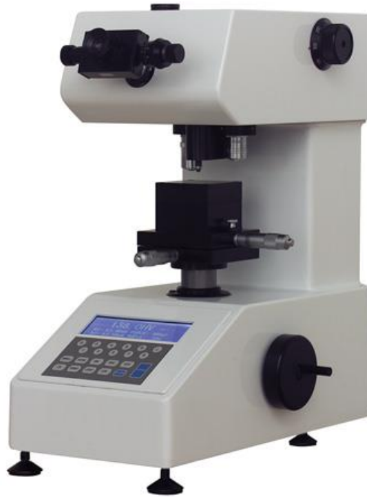
Figure 6 A commercial Vickers HMV microhardness tester (Shimadzu, Japan) comprising of the eyepiece, indenter translation stage and display screen.
