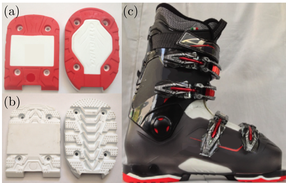
Figure 1: Samples of (a) design 1 sole and (b) design 2 sole and (c) ski boot used for the evaluation of the grip performance of the soles in the ramp test.
