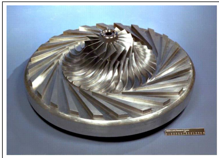
Figure 6-1: NASA CC3 compressor [116]
