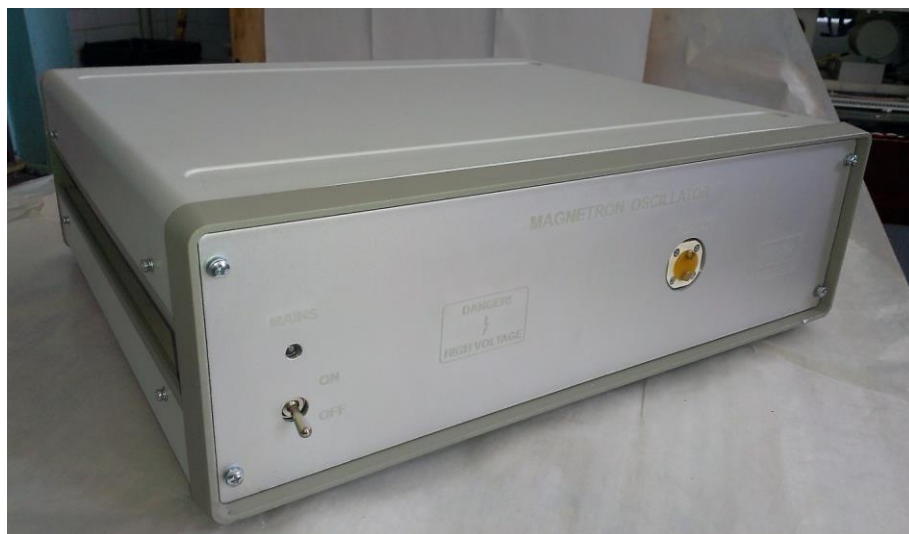
Figure 4.9 Photograph of a transmitter based on 95 GHz SHM.
