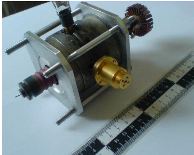
Figure 5.21 The photograph of the 210GHz magnetron (150mm*75mm*75mm, 1.3kg) [75].
