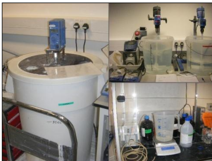
Figure 2.1 – Experimental set up for the manufacture of HA/SA Powder (Pilot plant in Apatech ltd)
