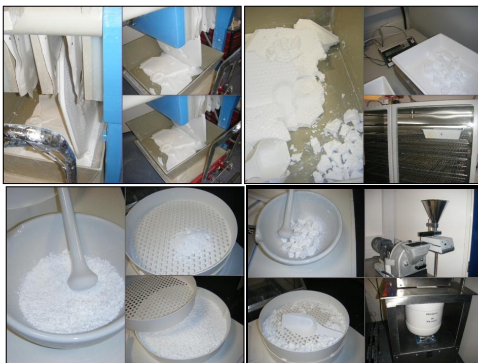
Figure 2.2 – Visual scheme of the filtering, drying, disc milling process of the powder
