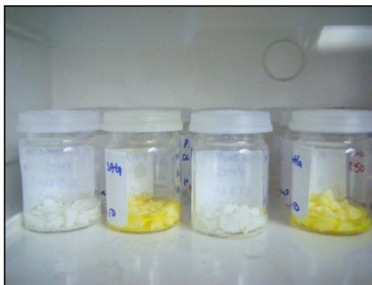
Figure 5.1 – Porous Granules of SA and HA submerged in physiological (300 ng/mL) and pharmacological (4 \mu\text{g/mL} ) concentrations of FTCA-rhBMP-2
