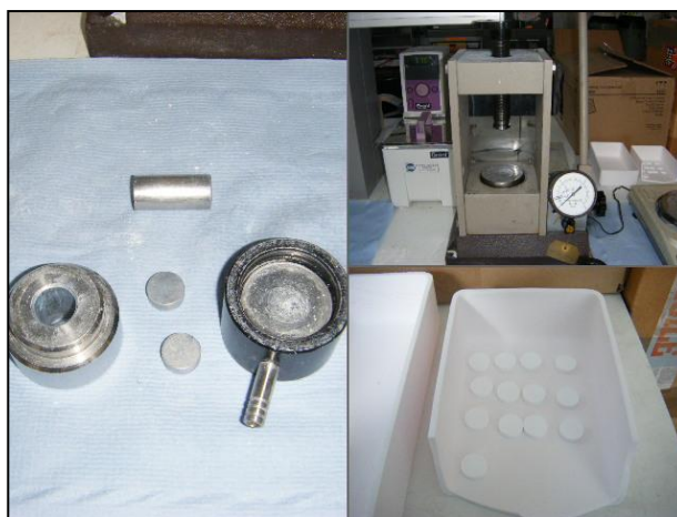
Figure 2.4 – Visual scheme of the compressing of biomaterial powder into DD
