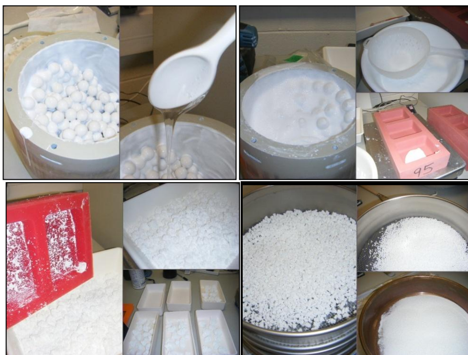
Figure 2.3 – Visual scheme for the foaming process for the production of PG
