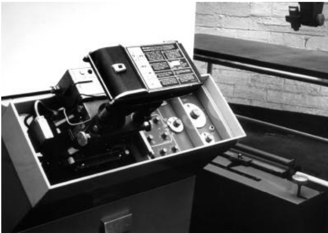
Figure 14. Control panel of the Disonograph – industrial design by Dugald Cameron. The most frequently used controls are in the extreme right-hand section: from the top – frequency selector, power switch and transmitter attenuator. The large dial in the centre section was used to set the mode of operation: B-scan, A-scan and inverted A-scan (for echo-encephalography), or M-mode. The other controls in this area are related to these modes of operation. At the left is a camera fitted with a Polaroid™ film back and an information projector to allow recording of patient data together with frequency and sensitivity settings, directly onto the film. A set of controls for occasional adjustment by an engineer are behind the hinged panel below the main control panel. This could be opened by the handle at the bottom of the picture.
