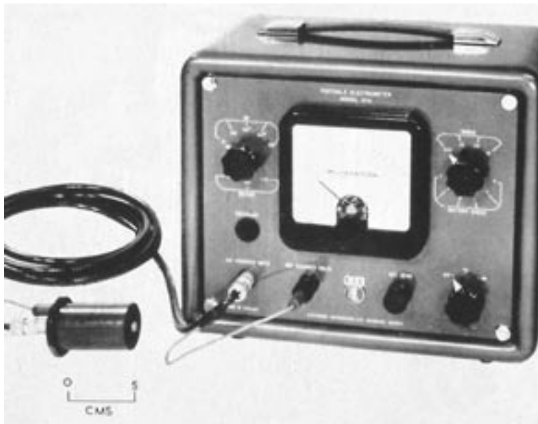
Figure 6: X-ray dosemeter and ion chamber used by the Adrian Committee Survey of Gonad Dose, developed by Sidney Osborn. See Stewart and Osborn (1959): 105; Osborn and Borrows (1958).
