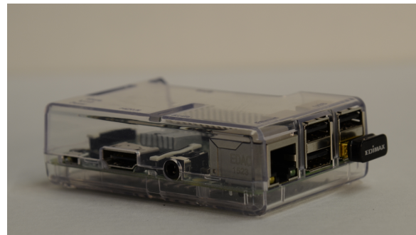
Figure 1: The MusicBox runs on a Raspberry Pi B. The system is configured to work as an open access point. Mobile devices connect to the MusicBox and start the web application with their browser. Once connected, the timing between the mobile device and the MusicBox is synchronized. The mobile device is then part of the musical space.
