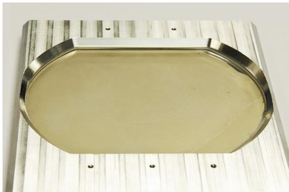
Fig. 9. Photographs (top) of the polished patterned copper on the quartz FSS substrate before attachment of the superstrate and (bottom) placeholder of the completed FSS in its mount.
