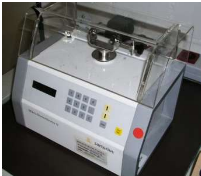
Figure 2.10: A dismembrator with cryotube attached, set at 2000 RPM for one minute to homogenise a sample into powder form, aiding complete homogenisation with Trizol.
