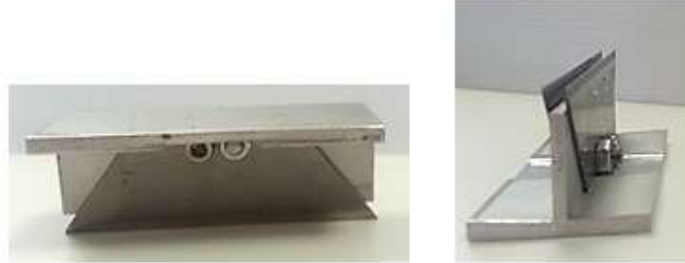
Figure 2.19: Picture of the custom-made membrane cutter. Dimensions - width 2mm, and length 14mm
