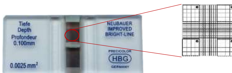
Figure 2.18: A haemocytometer – showing the grids in which cells are counted. All cells within the central grid, and those touching the top or left perimeter of the grid were counted, while those on the bottom or right perimeter were ignored.
