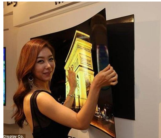
d) LG's 1.9kg 55-inch wallpaper thin White OLED TV poised on a magnetic wall mount (2015)
