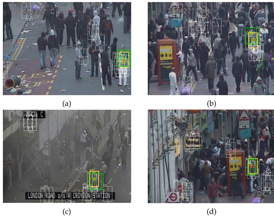
Figure 5.13: Visual comparison of pattern detection results from the same query as Figure 5.12, using the Hough-forest-based pattern index method described in this chapter. Green rectangles are ground truth, yellow rectangles show the detected area and white rectangles show lower-ranked detection positions, eliminated in preference for the yellow.
