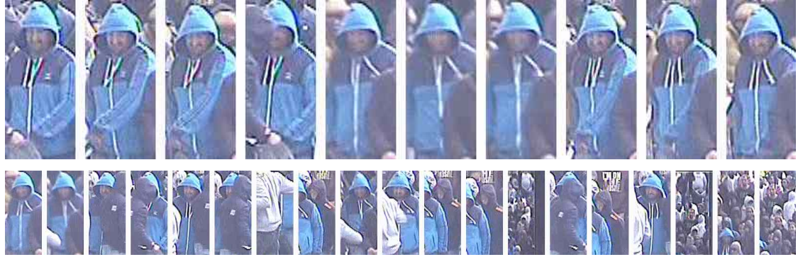
Figure 5.2: Tracked regions are extracted before and after the query frame. (a, Top) The 10 best matching regions are selected as positive training images ( n^{\oplus} = 10 ). (b, Bottom) Rejected candidate positive training images, based on the values of \gamma_r = 0.16 and \gamma_t = 0.1 . Images are sorted in descending \gamma_{m_i} ; varying n^{\oplus} will select more or fewer from the left of (b) into (a).
