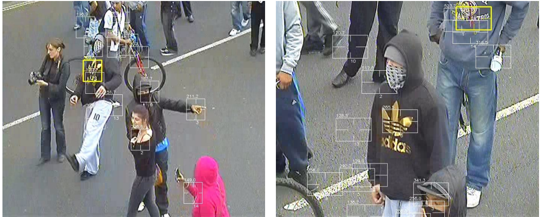
Figure 5.14: Result of searching for multiple patterns in one video using a single forest. Left, the adidas logo is correctly found, and Right, the marble hill logo is detected, shown with a yellow rectangle.
