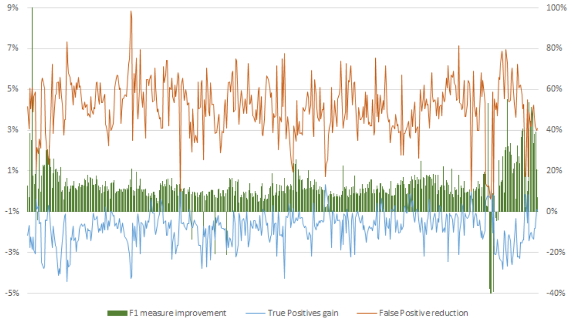
Figure 4.11: Difference in F_1 accuracy using only the Hue component on near-grey images. The slight reduction (2-4%) in True Positive values (blue) is compensated by a larger reduction (up to 9%) in the False Positive rate (orange). The overall F_1 measure is consistently improved in 92% of the 145 frames (green).
