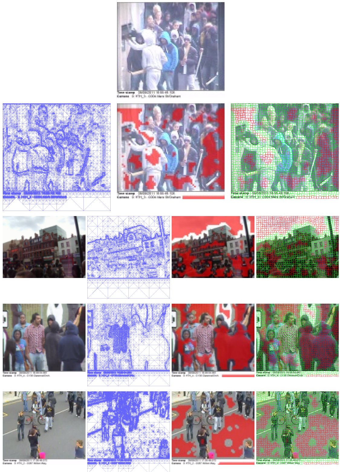
Figure 5.7: Triangular decomposition (column 2) searching for high-saliency areas. Negative training patches will be extracted from red regions in column 3, and positive training patches will be extracted from the unmarked regions. A randomly offset grid (column 4) of 16 \times 16 patches placed over the image are labelled green squares as positive training patch positions and red are used as negative training positions (based on intersection of the mask in column 3).
