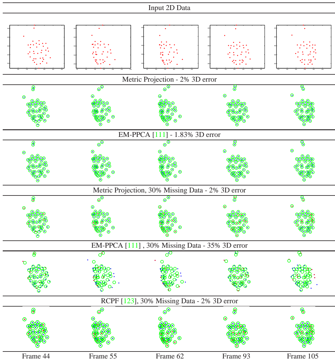
Figure 3.10: 3D reconstruction results for the “CMU” face motion capture sequence. First row: input 2D data. Second and third rows: full data results, Metric Projection and EM-PPCA. Reconstruction (blue dots) are compared with ground truth data (green circles). Fourth, fifth and sixth rows: Results for 30% missing data (highlighted in red).
