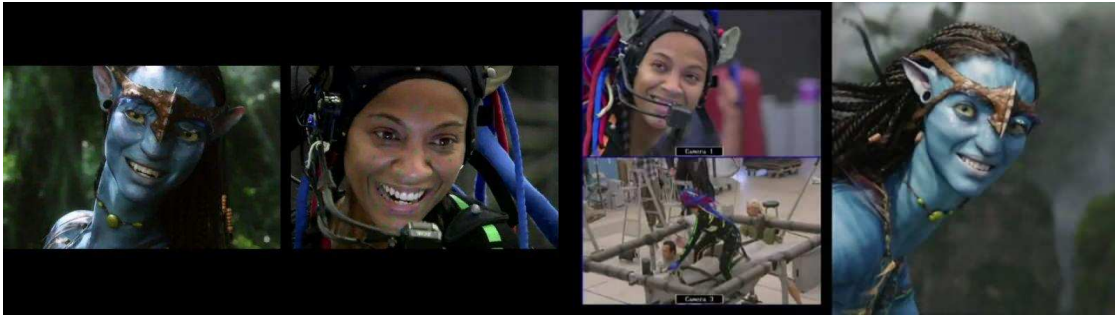
Figure 1.4: Motion capture systems applied in the movie industry: infrared markers are used together with a multi-camera system of infrared cameras to track the position of the body, while a camera focused on the face captures facial expressions, to be re-targeted on the 3D animation character. Images copyright Twentieth Century Fox.
