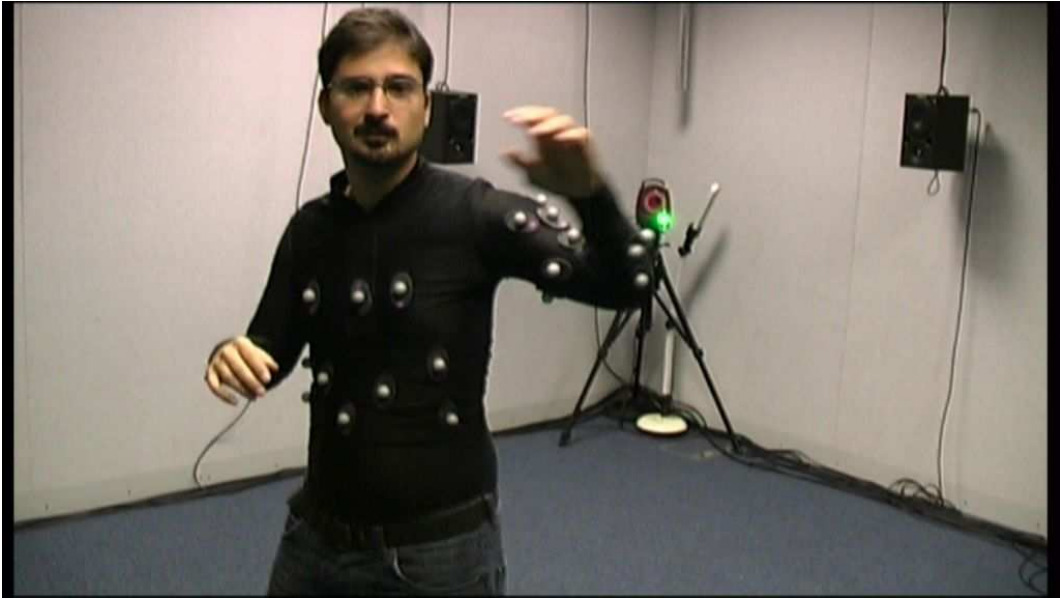
Figure 1.3: Motion capture with reflective markers require expensive infrared cameras and complicated setup
