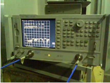
Fig. B 1. HP8720ES Vector Network Analyser used for on-body measurement.
