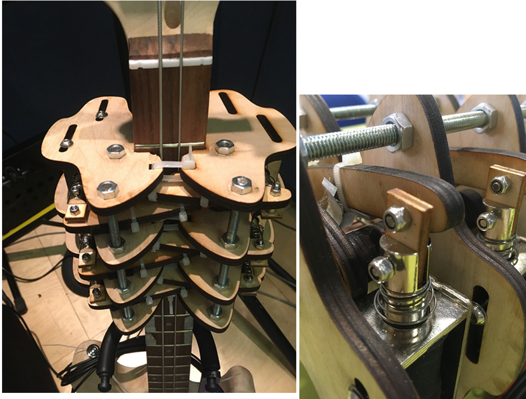
Figure 5: a) side view of neck clamp; b) solenoid plunger attachment to tip of fretting arm
