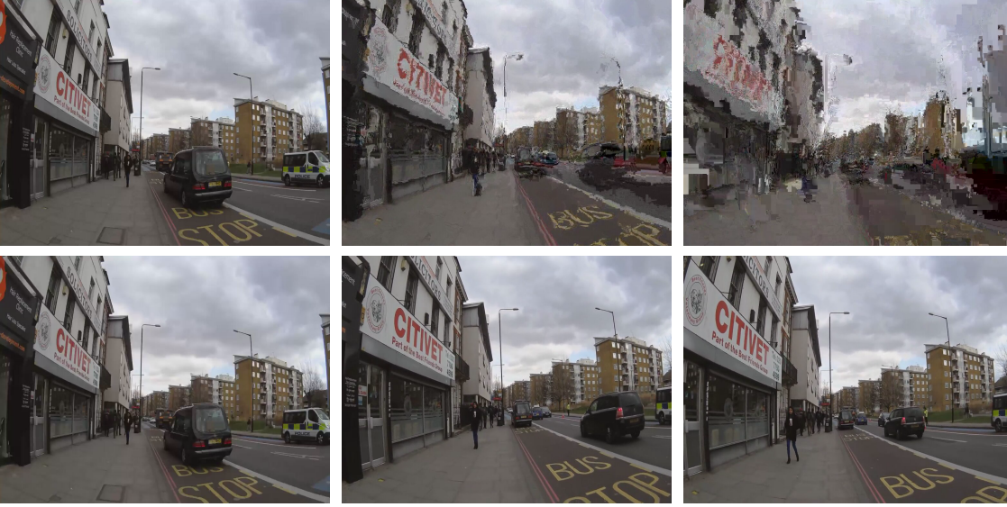
Figure 4.10: Sample frames captured at 2 s intervals representing received video quality with CBR 6 Mbit/s (first row) and our rate adaptive scheme (second row) for a multistream video multicast.
