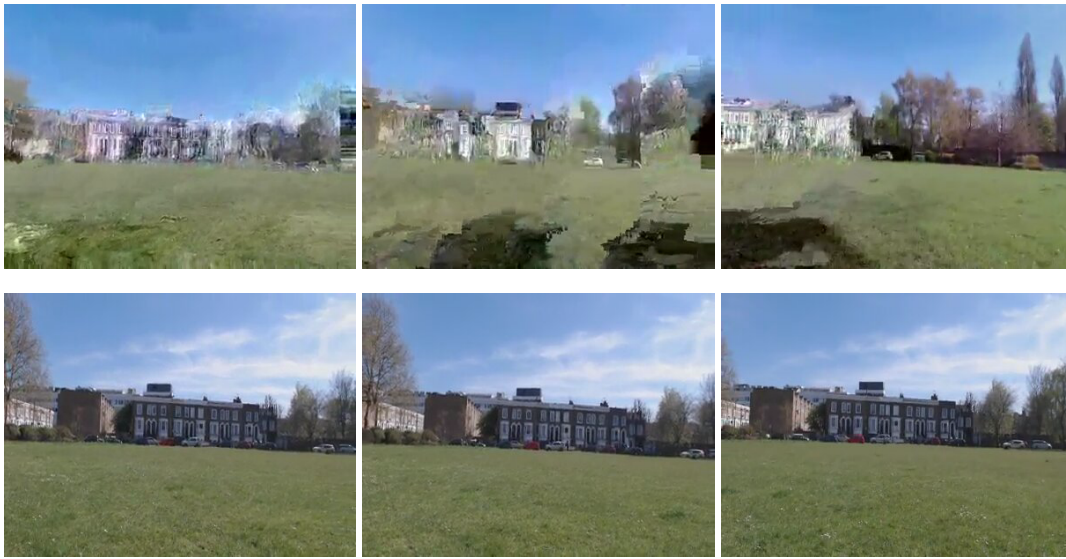
Figure 4.12: Sample frames representing received video quality with CBR 6 Mbit/s encoded at 128 kbit/s (top row) and our rate adaptive scheme (bottom row) for a multicast video stream.
