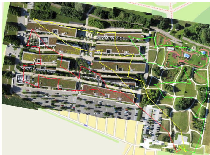
Figure 3.8: Overview image of the area of interest for coverage mission with three paths optimized to provide maximum aerial coverage
