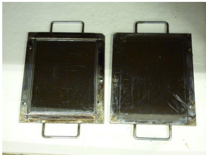
Figure 3-2. Mould used in the hot press to vulcanise 240mm x 200mm x 2mm sheets
