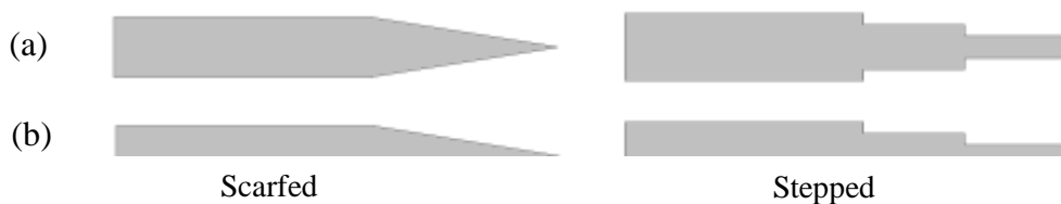
Fig.2.9 Metal parts of Comeld™ joints, (a) double-sided joints, (b) single-sided joints
