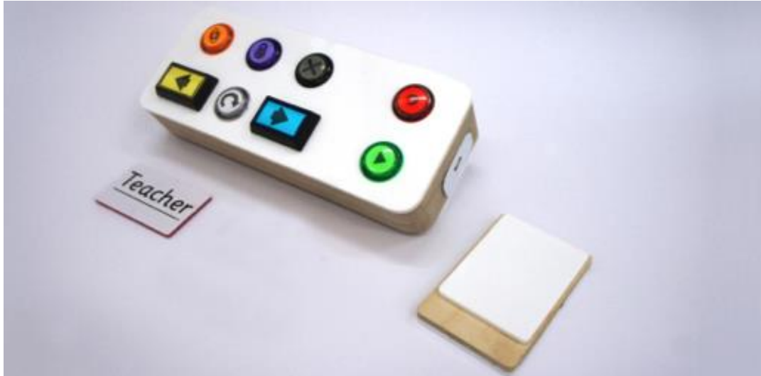
Figure 11 - Photo-sorting console with RFID card & reader
