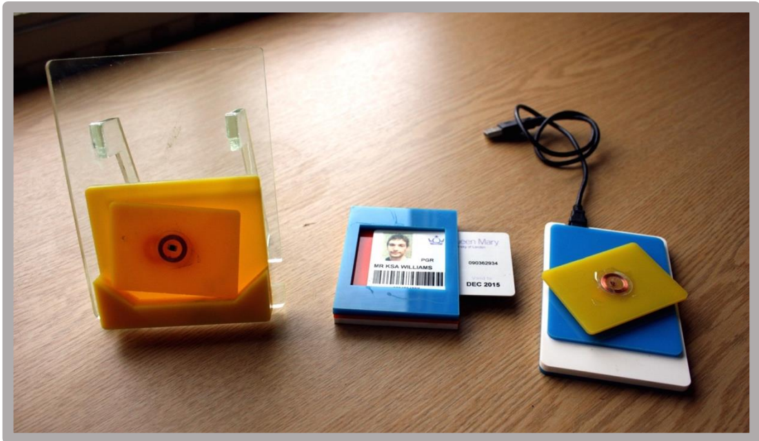
Figure 31 - Early prototype RFID reader designs (left and middle) and final design (right)
