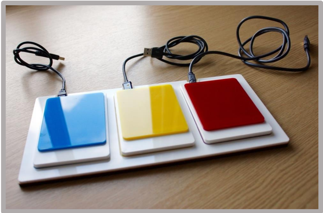
Figure 41 - Story game RFID readers. One reader for background image, one for the character and one for the sound effect
