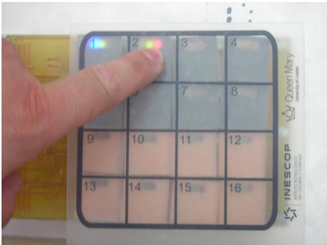
Figure 3.16. Specific device for Stroop test software (LED design).
