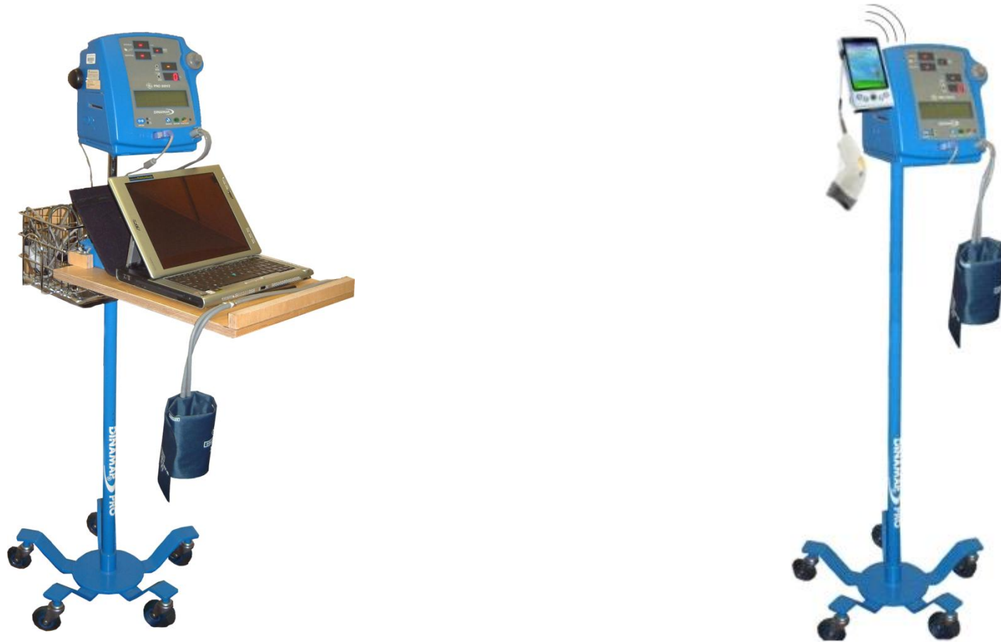
Figure 2.13. Hardware setup for Dinamap using a Tablet (left) and Pocket PC (right).
