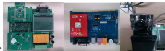
Fig. 2 Overview of CC2530 (left), GPS (middle) and camera (right)
