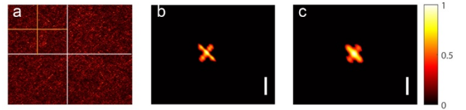
Fig. 5. Image reconstructions from a section of the raw speckle image. (a) The raw speckle image captured by the camera. (b) The reconstructed object calculated from the top left 1/4 section of the speckle image. (c) The reconstructed object image calculated from 1/16 section of the speckle image. Scale bar is 2mm, same as the object size.
