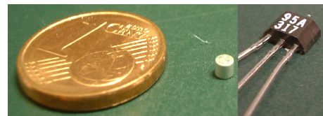
Fig. 3. Hall-effect sensor and magnet, near to a 1 euro cent coin (for size comparison).
