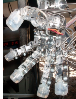
Fig. 1. Anthropomorphic robotic hand equipped with 12 tactile sensors.
