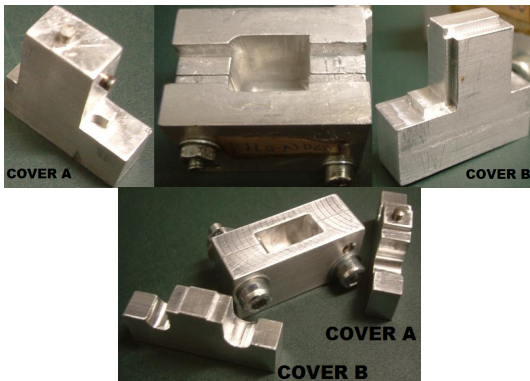
Fig. 6. Molds used to fabricate the silicone shells: top image, for the fingertip model, bottom image, for the phalangeal model.
