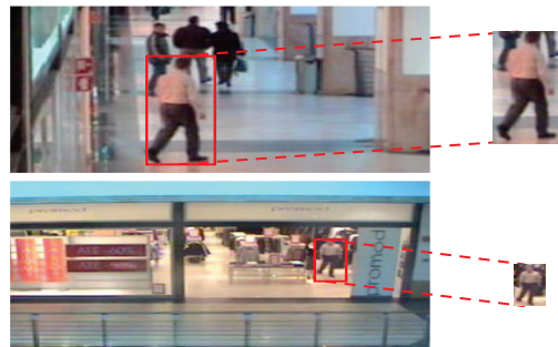
Figure 1. A typical person re-id scenario. The resolution of a person's images in two different camera views are significantly different, beyond the scope for simple image size normalisation by interpolation.
