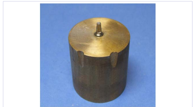
Figure 1a: Implant fixture and ITI Straumann Solid abutment embedded into brass cylinder also showing 2 location notches on brass cylinder to allow reproducibility.
