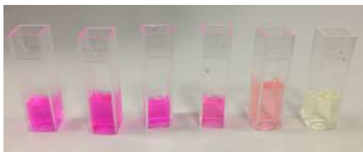
Figure 4.19 Sample dye solutions taken at different irradiation times for UV-Vis Spectroscopy
