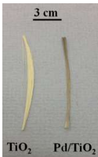
Figure 4.12 Colour change after Pd deposition on TiO 2 nanorods on glass fibre substrates
