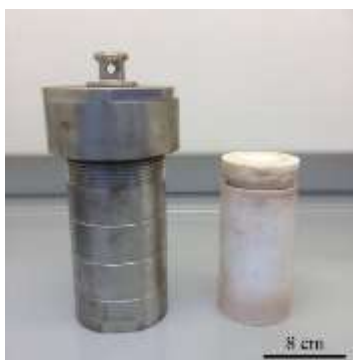
Figure 3.2 Teflon-lined stainless steel autoclave (Toption Group Co Ltd, China)
