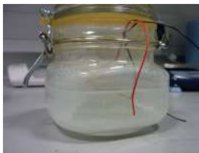
Figure 3.1 Sealed jars used for growing ZnO nanorods with an aqueous method
