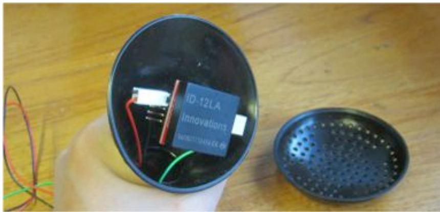
Figure 34: Detail of the watering can spout with ID-12 RFID reader inside
