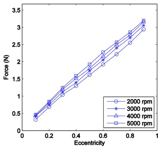
Figure 8 – Load magnitude plotted against eccentricity for a journal bearing with  $\Lambda = 0.85$  and  $C = 1.7$  at speeds from 2000 to 5000 rpm.
