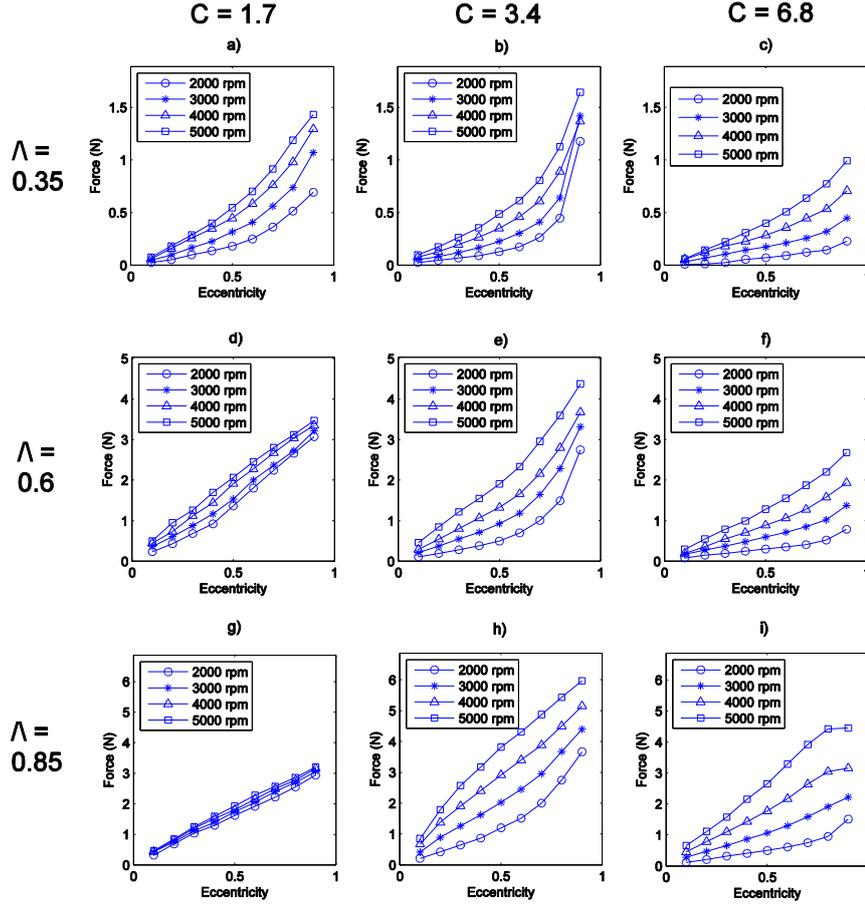
Figure 4 – Experimental results for the generated force with different journal bearings. a)  $C = 1.7$ ,  $\Lambda = 0.35$ . b)  $C = 3.4$ ,  $\Lambda = 0.35$ . c)  $C = 6.8$ ,  $\Lambda = 0.35$ . d)  $C = 1.7$ ,  $\Lambda = 0.6$ . e)  $C = 3.4$ ,  $\Lambda = 0.6$ . f)  $C = 6.8$ ,  $\Lambda = 0.6$ . g)  $C = 1.7$ ,  $\Lambda = 0.85$ . h)  $C = 3.4$ ,  $\Lambda = 0.85$ . i)  $C = 6.8$ ,  $\Lambda = 0.85$ .
