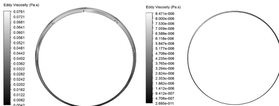
Figure 14 – Numerical solution for the eddy viscosity around the axial middle of the journal for a journal bearing with  $\Lambda = 0.85$ ,  $C = 6.8$  and  $\epsilon = 0.5$  at 5000 rpm (left) and  $\Lambda = 0.85$ ,  $C = 1.7$  and  $\epsilon = 0.5$  at 5000 rpm (right).
