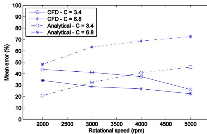
Figure 7 – Mean error for CFD and analytical solutions at various speeds.
