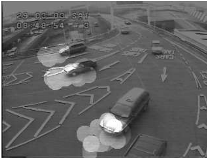
Figure 5.1: An example frame of the busy traffic scene computed using the accumulated temporal saliency algorithm. Temporally salient circular regions were accumulated over all relevant spatio-temporal locations. However, the temporally salient regions do not fully spatially overlap the moving objects.
