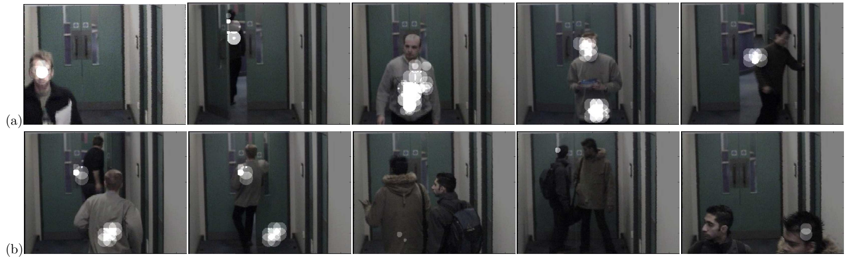
Figure 4.9: Frames illustrating the ranked top 10% least frequent co-occurrence elements from a corridor and entrance scene using the basic method from Eqn. (4.3). Co-occurrences at particular spatial locations are highlighted with circles. Sizes of the circles indicate the scale at which the entropy peaks within that local spatio-temporal neighbourhood and their intensity represents the temporal saliency where lighter shades represents higher values.
