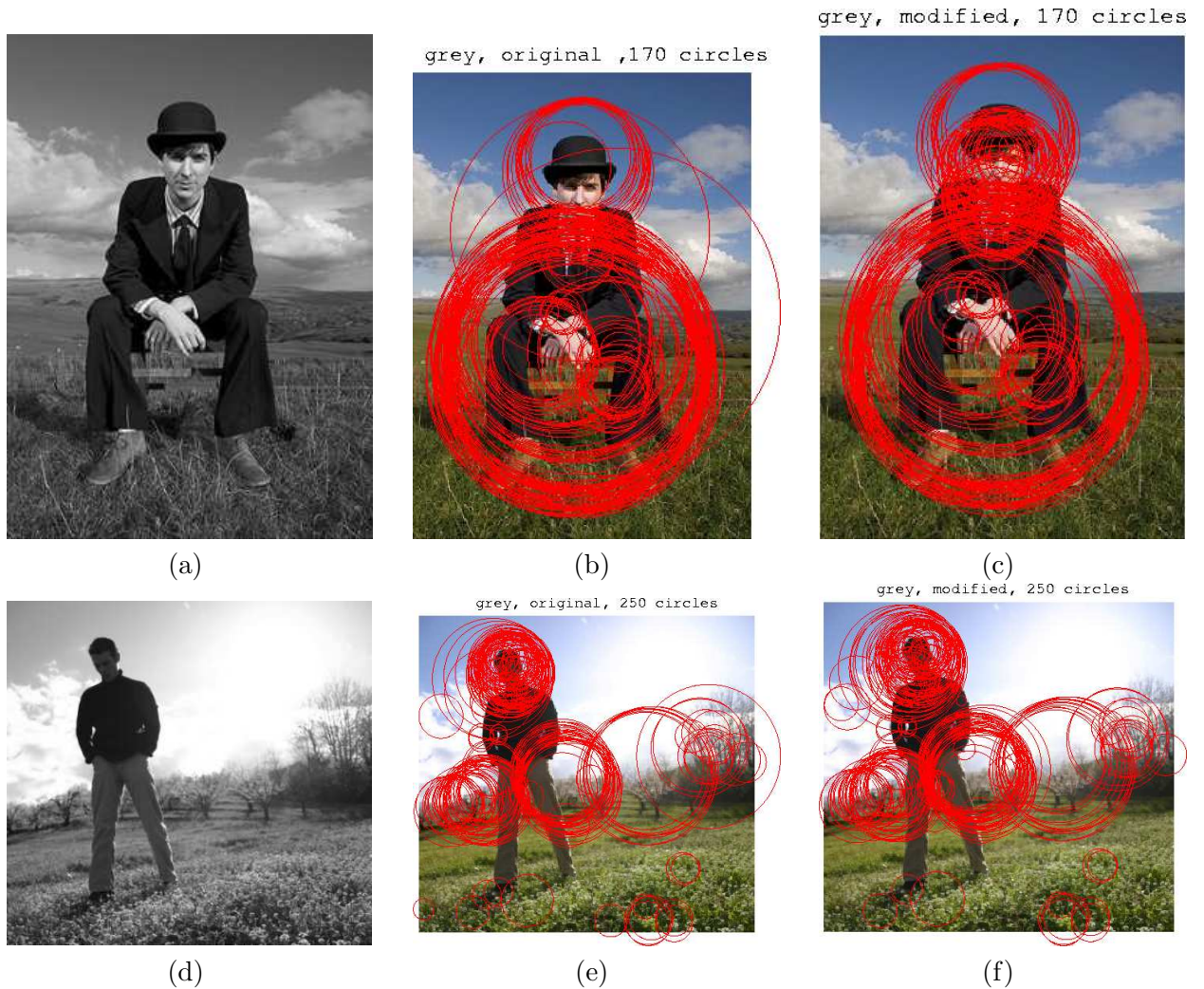
Figure 3.3: Further comparison between Kadir and Brady’s original method and the modification in Equation 3.7-3.8. The first column shows the original image, the middle column shows results using the original scale saliency algorithm and the right-most column shows results using the modified version. The circles show the top N most spatially salient regions where the size of the circles indicates the salient spatial scale. The images used in the two result columns are shown in colour for easier discrimination between that and the salient spatial regions marked with red circles.
