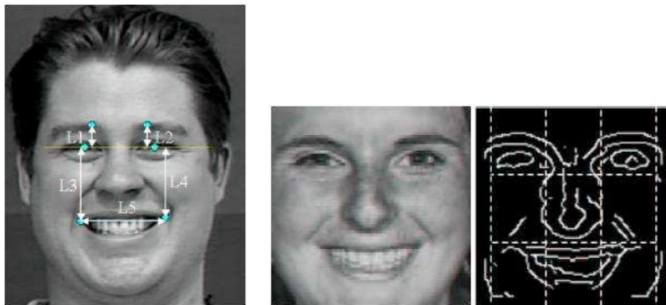
Figure 2.5: Geometric features [153]: ( Left ) location features; ( Right ) normalized face and zones of the edge map of the normalized face.
