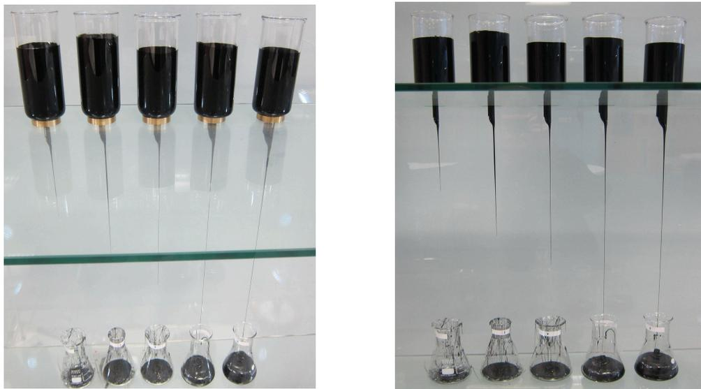
FIG. 1: Experimental setup showing top and bottom views of glass tubes with flowing bitumen. The radius of orifices increases from left to right.
