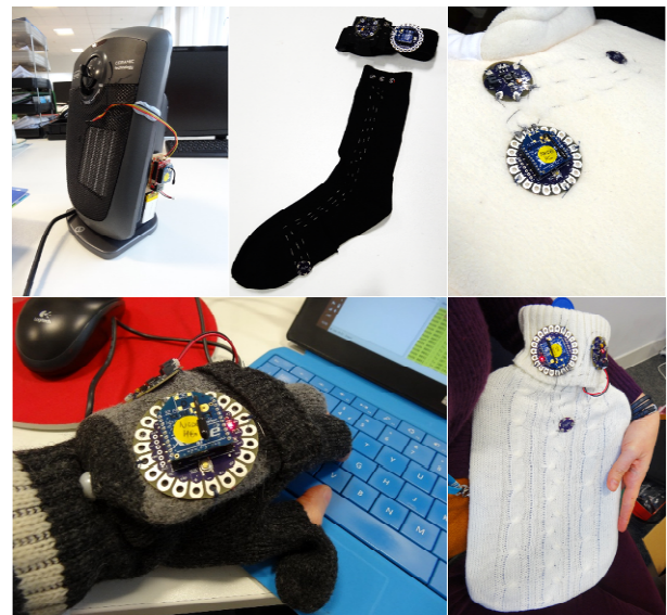
Figure 3.1: Personal Heating Devices, clockwise from top left: personal fan heater, heated socks, heated shoulder pad, heated gloves, and hot water bottle.
