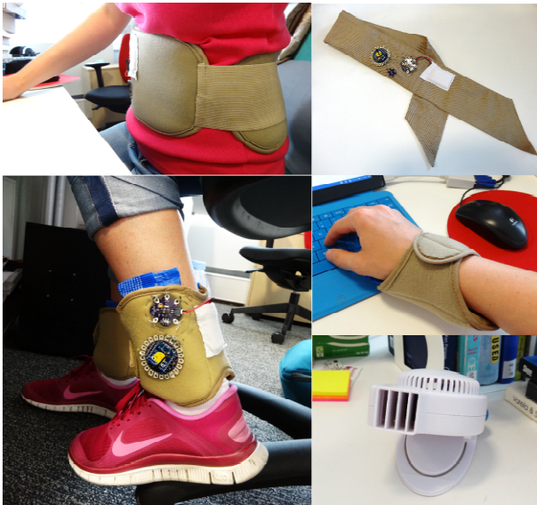
Figure 3.2: Personal Cooling Devices, clockwise from top left: cooling body wrap, cooling neck tie, wrist cooler, personal cooling fan, and ankle coolers.
