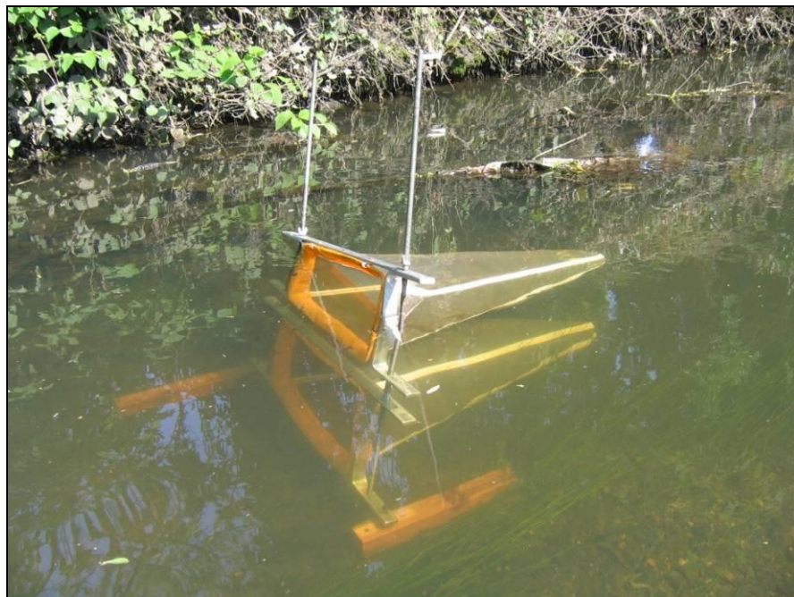
Figure 6.4: Drift nets mounted on a frame (top) and sampling in the river (above).
