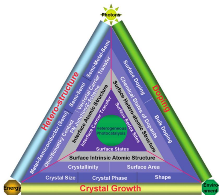
Figure 2.7 The relation between crystal growth, doping and heterostructure in semiconductor photocatalysis (adapted from Liu et al., 2010) 14
