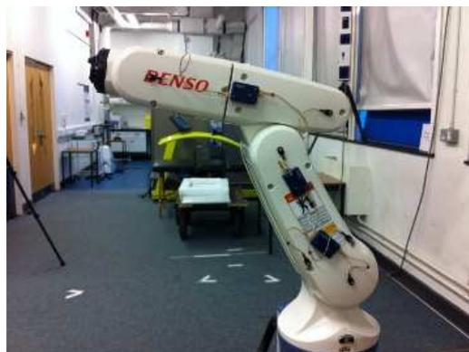
Fig. 1. The configuration of markers on the robot arm that was used on both sides of each segment. The large black boxes contain the batteries and electronics.
