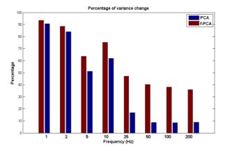
Fig. 3. Percentage of variance change for different frequencies before and after applying PCA and F-PCA based signal separation techniques.
