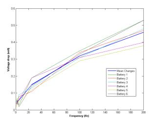
Fig. 2. Voltage drops in sensors batteries versus frequency of sampling.
