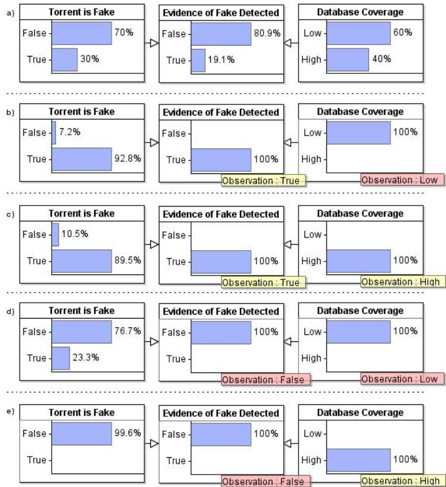
Figure 14: Possible Outcomes of the Fakes Detection Model: a) Show the marginal values before propagation, b-e) Show the values after propagation with the given observations
