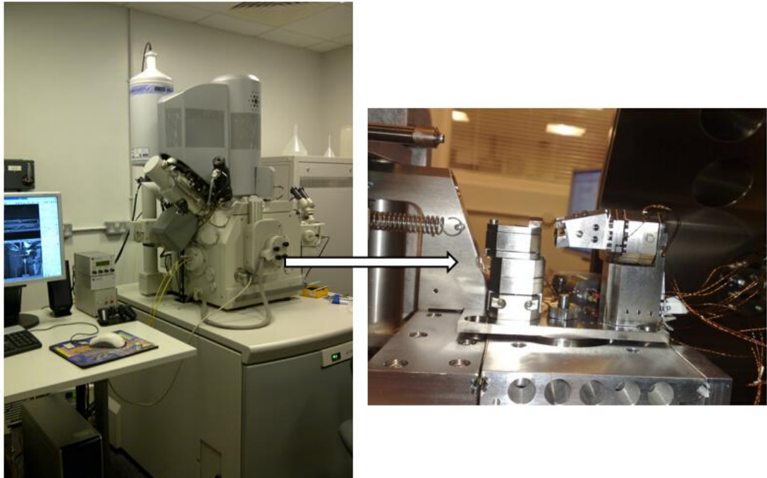
Figure 1.1 Photographs highlighting the experimental setup used to combine SEM, FIB and AFM techniques within a single instrument. The left image shows a standard SEM-FIB dual-beam system (Quanta 3D FEG, FEI, USA/EU) whereas the right image indicates a custom built AFM that sits inside the SEM vacuum chamber and therefore allows in situ mechanical testing of small volumes of a wide range of biological samples.
