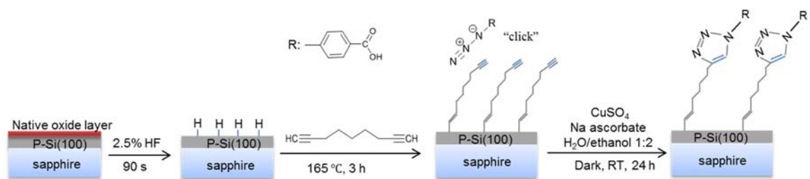
Figure 1 Modification of 1,8-nonyne monolayers on SOS substrates using "click" cycloaddition to generate \text{CO}_2\text{H} -terminated monolayers.
