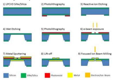
Fig. 7 Proposed fabrication process
