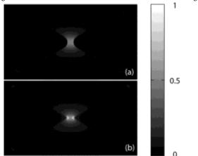
Fig. 4. Normalized electric field distributions of (a) a round bowtie and (b) an ideal bowtie
