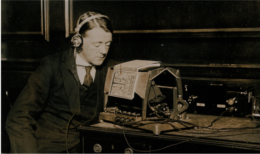
Figure 2 A blind man reading a book using the Optophone. Wellcome Library, London.
