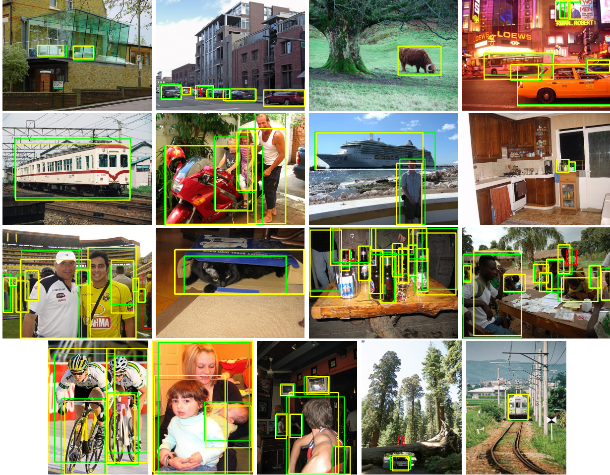
Figure 3. Qualitative examples of our edge grouping based objectness measure. An IoU threshold of 0.65 is used to determine if correctly discover an object here. Yellow boxes are the best produced candidates of our method. Ground truth bounding boxes are shown in green and red, while green indicates correctly discovering an object and red indicates failure of the detection.
