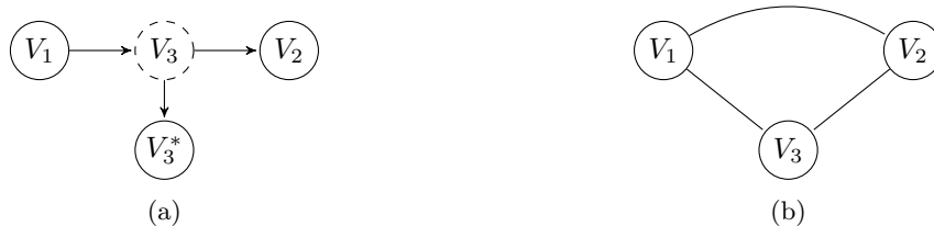
Figure 4.4: (a) A noisy graph that contains three error-free variables V_1, V_2 and V_3 , and a noisy variable V_3^* . (b) The learnt graph that entails the same dependence and independence relationships derived from the observed variables.
