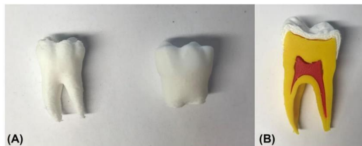
Fig. 4. 3D printed mandibular first molar (A) both natural and artificial molar in PLA and (B) natural molar in multiple materials, PLA for enamel, TPE for dentine and pulp cavity.
