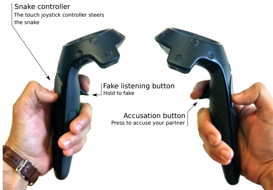
Figure 4.2: The user interface includes buttons to start and stop faking, accuse others for faking, and control the snake game while faking.
