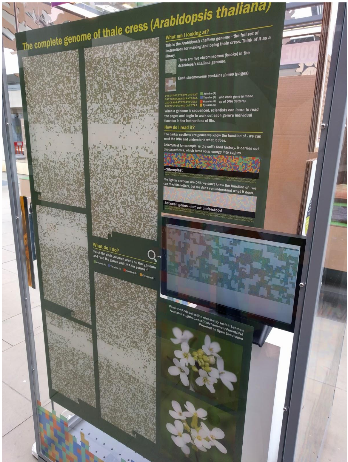
Figure Supplemental-1.1: Final poster displayed in the Millennium Seed Bank. The left two thirds of the poster are backed by Displax touch sensitive film (visible as an orange strip on the far left) for user input. On the right, an embedded computer monitor running FluentDNA with a digital copy of the poster. Touching the poster causes the monitor to zoom in on the corresponding place in the genome and display the sequence and function of the gene that was touched.
