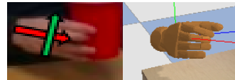
Fig. 2. Our manually defined red directional vector and green up vector (left). The blue right vector is obtained as the vector orthogonal to both the directional and up vector. The reconstructed hand model (right).
